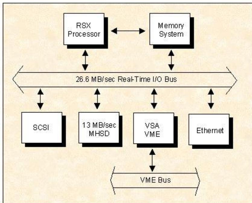
Figure 3. Real-Time I/O Bus
