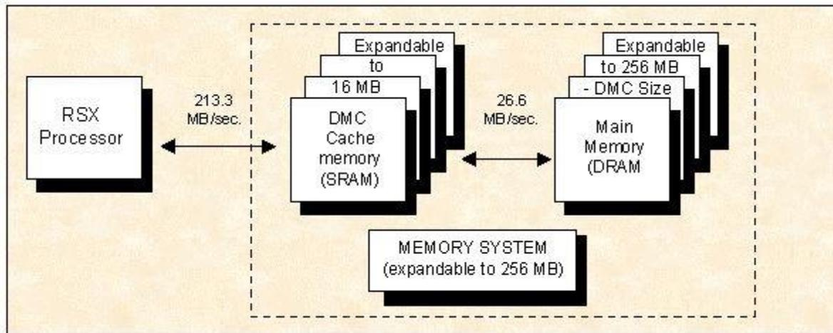
Figure 2. CPU/Cache/Memory System Design
